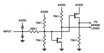
FIGURE 45. TRI-LEVEL DIGITAL INPUTS
