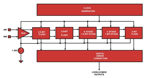
FIGURE 22. A/D CORE BLOCK DIAGRAM
