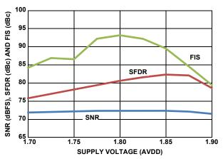
FIGURE 21. ANALOG SUPPLY VOLTAGE SWEEP WITH I2E FROZEN, I2E PREVIOUSLY CALIBRATED AT 1.8V,  $F_{\text{IN}}$  = 105MHz
