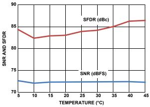
FIGURE 25. TYPICAL SNR, SFDR PERFORMANCE vs TEMPERATURE, DEVICE CALIBRATED AT +25  $^{\circ}$  C, 500MSPS OPERATION,  $f_{\rm IN}$  = 105MHz
