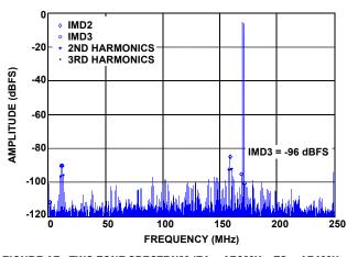
FIGURE 17. TWO-TONE SPECTRUM (F1 = 170MHz, F2 = 171MHz -7dBFS)
