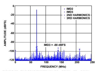
FIGURE 16. TWO-TONE SPECTRUM (F1 = 70MHz, F2 = 71MHz -7dBFS)
