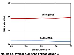
FIGURE 26. IYPICAL SNK, SFDR PERFORMANCE VS TEMPERATURE, DEVICE CALIBRATED AT +85°C, 500MSPS OPERATION,  $f_{\rm IN}$  = 105MHz
