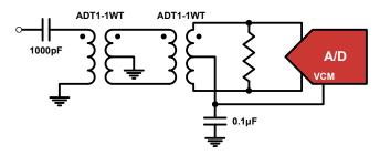
FIGURE 28. TRANSFORMER INPUT FOR GENERAL PURPOSE APPLICATIONS
