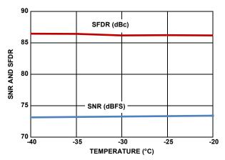
FIGURE 24. TYPICAL SNR, SFDR PERFORMANCE vs TEMPERATURE, DEVICE CALIBRATED AT -40  $^{\circ}$  C, 500MSPS OPERATION, f<sub>IN</sub> = 105MHz
