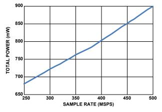
FIGURE 8. POWER vs  $f_{\mbox{SAMPLE}}$  IN 3mA LVDS MODE
