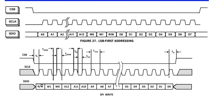
FIGURE 38. SPI WRITE
