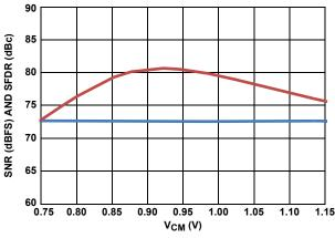
FIGURE 11. SNR AND SFDR vs  $V_{CM}$
