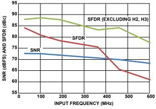
FIGURE 2. SNR AND SFDR vs  $f_{\mbox{\scriptsize IN}}$
