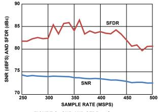
FIGURE 6. SNR AND SFDR vs f<sub>SAMPLE</sub>
