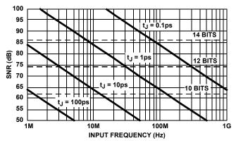
FIGURE 32. SNR vs CLOCK JITTER
