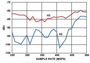
FIGURE 7. HD2 AND HD3 vs f<sub>SAMPLE</sub>
