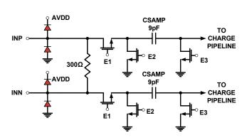
FIGURE 43. ANALOG INPUTS
