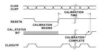
FIGURE 23. CALIBRATION TIMING
