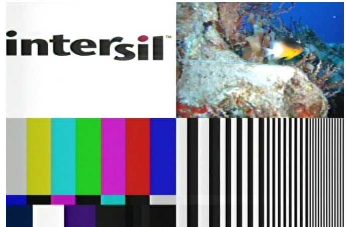
FIGURE 42. TEST PATTERN IMAGE AFTER 6000 FEET OF RG-59 COAX WITH ISL59603 (OR BETTER)
