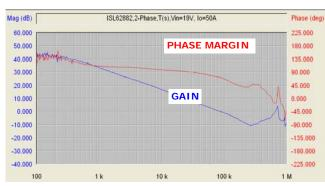
FIGURE 51. 2-PHASE CPU MODE REFERENCE DESIGN LOOP GAIN T2(s) MEASUREMENT RESULT
