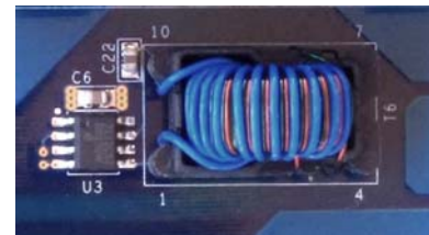
FIGURE 9. PULSE TRANSFORMER AND DRIVER
