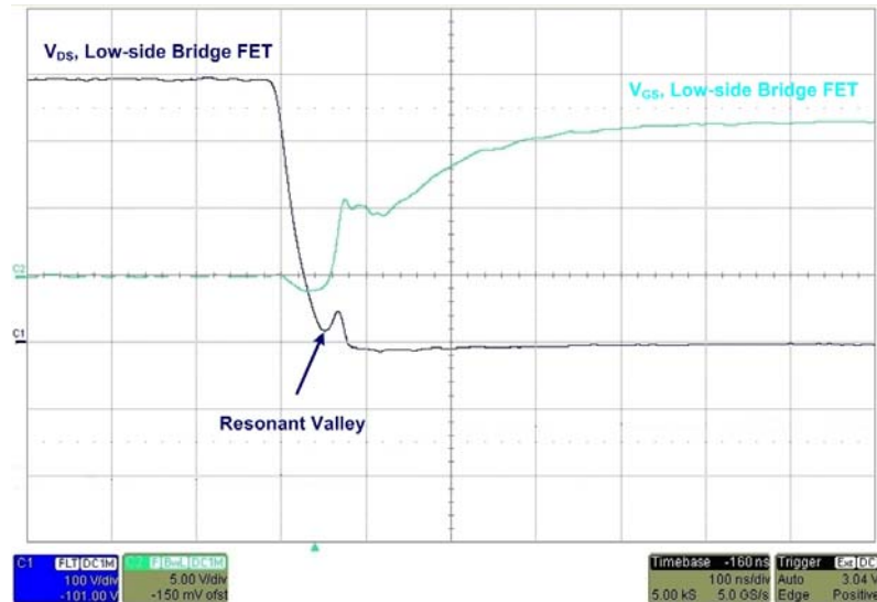
FIGURE 21. RESONANT SWITCHING WITH 100% (50A) LOAD
