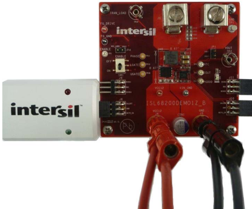
FIGURE 5. ISL68200 DEMONSTRATION BOARD SETUP
