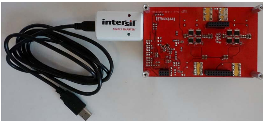
FIGURE 9. ISL78229EV1Z CONNECTED TO INTERSIL DONGLE FOR GUI (BOTTOM VIEW)
