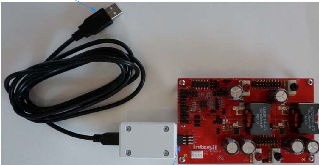
FIGURE 8. ISL78229EV1Z CONNECTED TO INTERSIL DONGLE FOR GUI (TOP VIEW)
