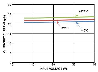
FIGURE 4. QUIESCENT CURRENT vs INPUT VOLTAGE (NO LOAD)
