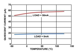
FIGURE 2. QUIESCENT CURRENT vs LOAD CURRENT (AT UNITY GAIN),  $V_{\rm IN} = 14V$
