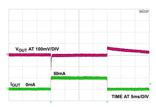
**FIGURE 9. LOAD TRANSIENT RESPONSE**
