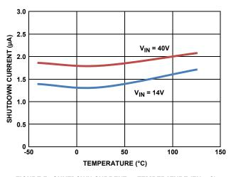
FIGURE 5. SHUTDOWN CURRENT vs TEMPERATURE (EN = 0)
