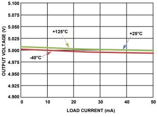
FIGURE 7. OUTPUT VOLTAGE vs LOAD CURRENT
