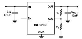
FIGURE 14. SETTING OUTPUT VOLTAGE
