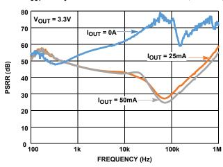
FIGURE 10. PSRR vs FREQUENCY FOR VARIOUS LOAD CURRENT,  $V_{OUT} = 3.3 \text{V} \label{eq:voltage}$
