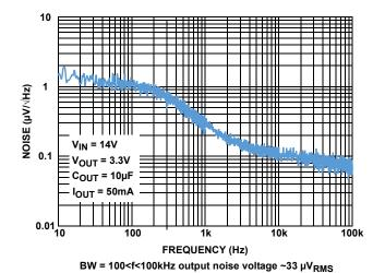
FIGURE 13. OUTPUT NOISE SPECTRAL DENSITY, I<sub>OUT</sub> = 50mA
