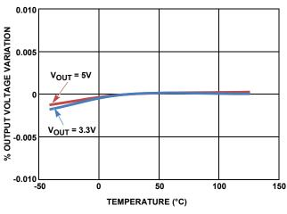
FIGURE 6. OUTPUT VOLTAGE vs TEMPERATURE (LOAD = 50mA)
