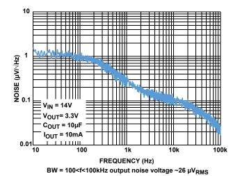
FIGURE 12. OUTPUT NOISE SPECTRAL DENSITY, I<sub>OUT</sub> = 10mA
