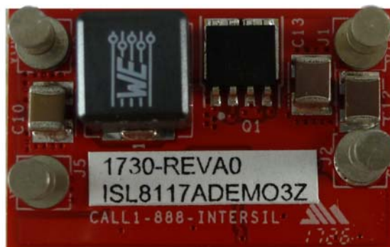
Figure 5. ISL8117ADEMO3Z Bottom Side
