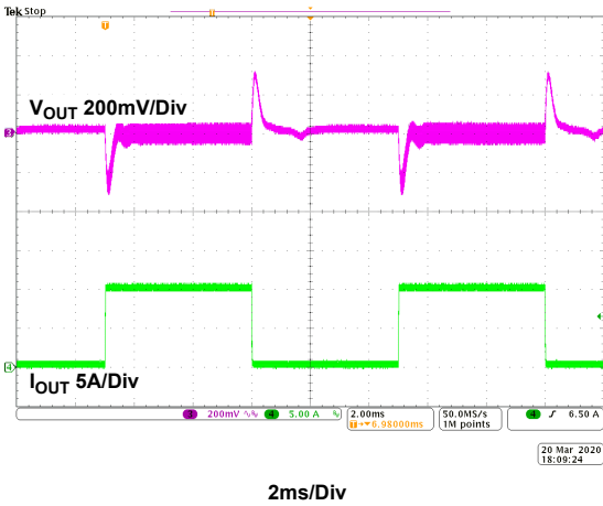
Figure 22. Load Transient, V_{IN} = 12V , I_{OUT} = 0A to 10A , 2.5A/\mu s , CCM
