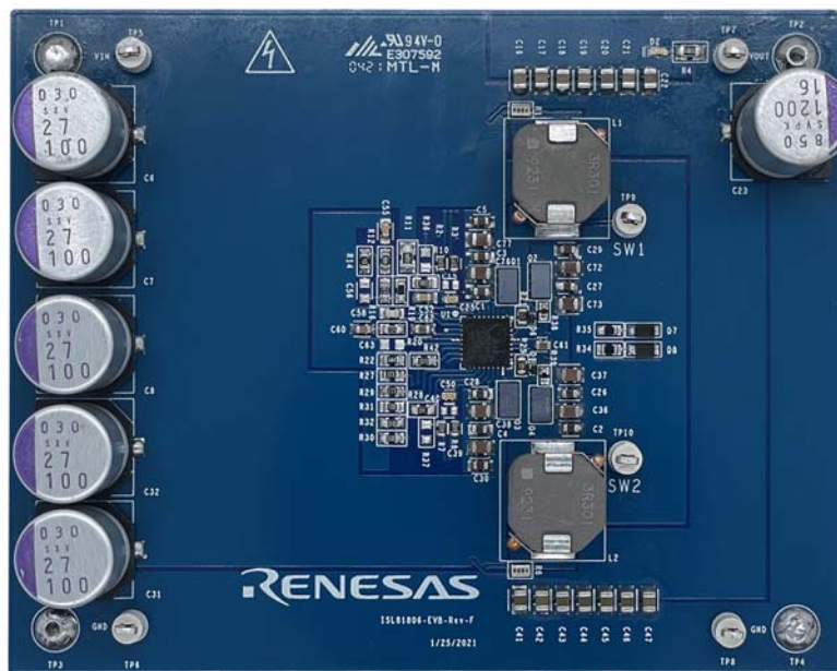
Figure 4. ISL81806EVAL1Z Evaluation Board, Top View
