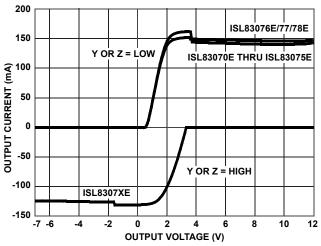
FIGURE 9. DRIVER OUTPUT CURRENT vs SHORT CIRCUIT **VOLTAGE**
