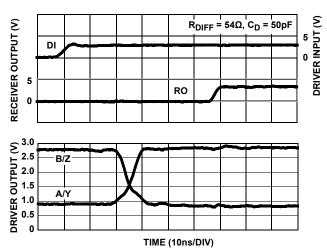
FIGURE 21. DRIVER AND RECEIVER WAVEFORMS, LOW TO HIGH (ISL83076E, ISL83077E, ISL83078E)
