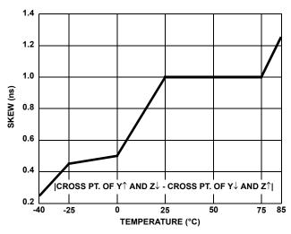
FIGURE 14. DRIVER DIFFERENTIAL SKEW vs TEMPERATURE (ISL83073E, ISL83075E)
