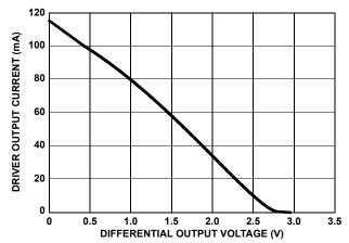
FIGURE 7. DRIVER OUTPUT CURRENT vs DIFFERENTIAL **OUTPUT VOLTAGE**
