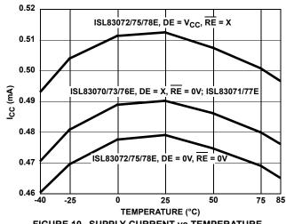
FIGURE 10. SUPPLY CURRENT vs TEMPERATURE
