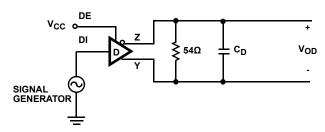
FIGURE 4A. TEST CIRCUIT
