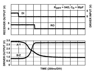
FIGURE 20. DRIVER AND RECEIVER WAVEFORMS, HIGH TO LOW (ISL83073E, ISL83075E)
