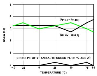
FIGURE 13. DRIVER SKEW vs TEMPERATURE (ISL8490E/ISL8491E)
