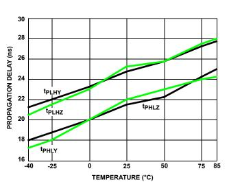
FIGURE 12. DRIVER PROPAGATION DELAY vs TEMPERATURE (ISL8490E/ISL8491E)
