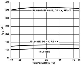
FIGURE 9. SUPPLY CURRENT vs TEMPERATURE
