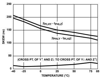
FIGURE 11. DRIVER SKEW vs TEMPERATURE (ISL8488E/ISL8489E)
