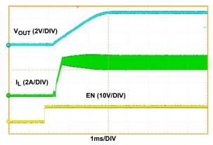
FIGURE 9. START-UP WITH EN, IOUT = 5A
