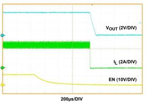
FIGURE 10. SHUTDOWN WITH EN, IOUT = 5A
