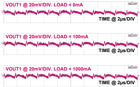
FIGURE 23. PWM1 OUTPUT RIPPLE, MODE = 5V (CCM)
