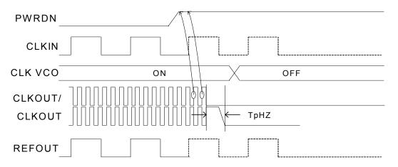
CLKOUT is driven differentially when PWRDWN# is de-asserted unless the CLKOUT is disabled through the SMBus register bit.
