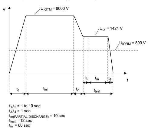
Method b) Non-destructive Test, 100 % Production Test
