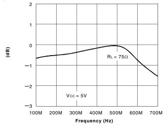
Insertion Loss vs. Frequency
