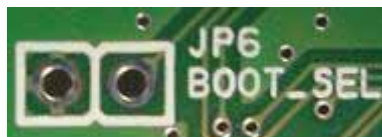
Figure 11 Switch Jumper (JP6) Serial Writer Function
