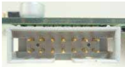
Figure 8 Connector for E8a Emulator (CN6)
