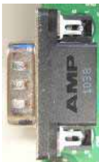
Figure 10 D-sub9 Pin Male Connector (CN5)
