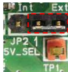
Figure 5 JP2 5V-dedicated power supply switch “Internal input (int)” setting “External input (Ext)” setting
