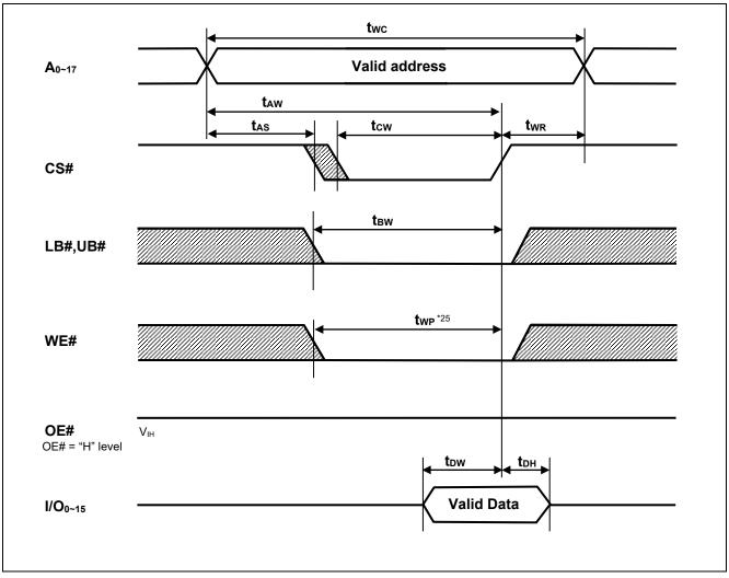
Note 25. twp is the interval between write start and write end.
