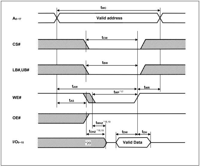
Note 17. twp is the interval between write start and write end.
