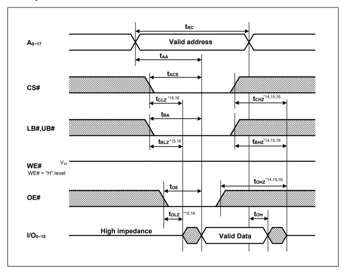
Note 14.  $t_{CHZ}$ ,  $t_{BHZ}$  and  $t_{OHZ}$  are defined as the time when the I/O pins enter a high-impedance state and are not referred to the I/O levels.
