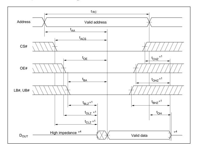
Read Timing Waveform (2) (WE# =  $V_{_{I\!H}},$  LB# =  $V_{_{I\!L}},$  UB# =  $V_{_{I\!L}})$
