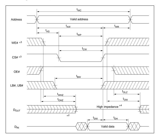
Write Timing Waveform (3) (LB#, UB# Controlled, OE# =  $V_{HH}$ )
