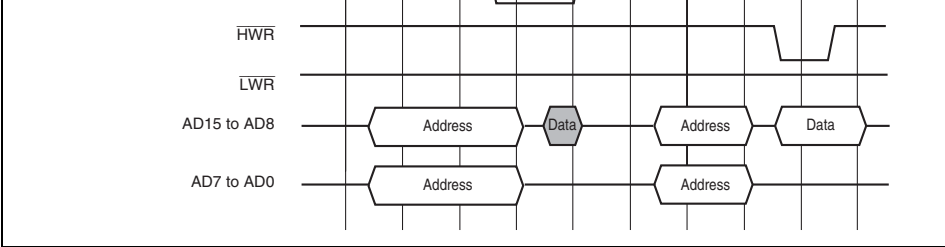
Figure 6.20 Bus Timing for 16-Bit, 2-State Access Space (2) (Even Byte Access)
