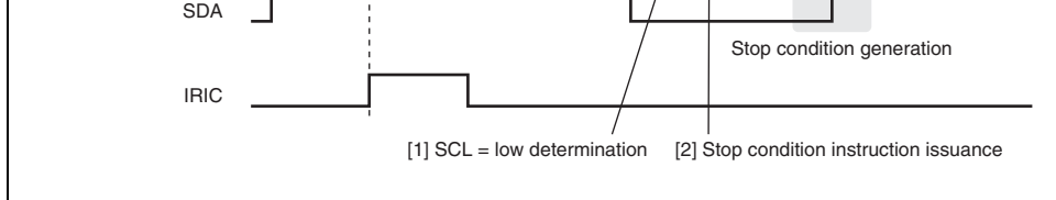
Figure 18.31 Stop Condition Issuance Timing
