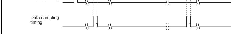
Figure 13.25 Receive Data Sampling Timing in Smart Card Interface Mode (When Clock Frequency is 372 Times the Bit Rate)
