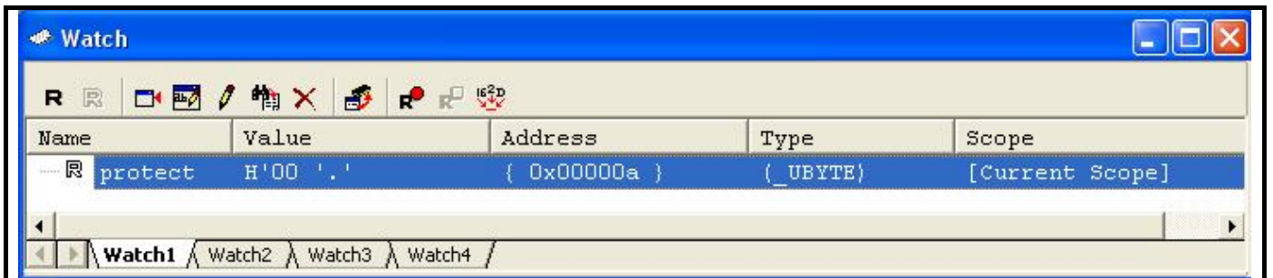
Figure 6.14 [Watch] Window (Array Display)
