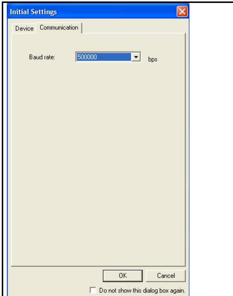
Figure 4.20 [Initial Settings] Dialog Box ([Communication] Tab)
