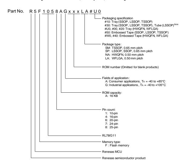
**Note** The packaging specification is only "Tube" for products in the 20-pin LSSOP.
