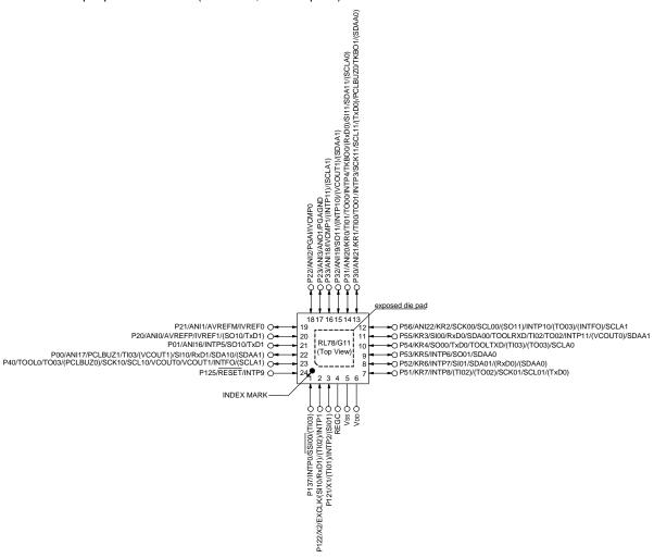
Caution Connect the REGC pin to Vss pin via a capacitor (0.47 to 1  $\mu$ F).
