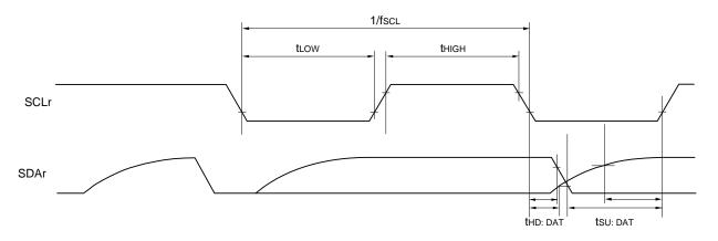
$\textbf{Remark 1.} \ \ Rb[\Omega]: Communication line (SDAr) \ pull-up \ resistance, \ Cb[F]: \ Communication \ line (SDAr, SCLr) \ load \ capacitance$
