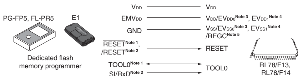
Figure 30-2. Communication with Dedicated Flash Memory Programmer
