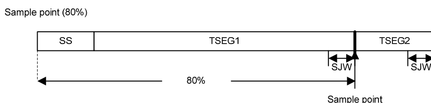
Figure 18-17. Bit Timing Chart
