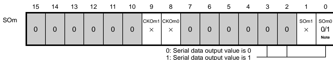
(e) Serial output register m (SOM) ... Sets only the bits of the target channel.
