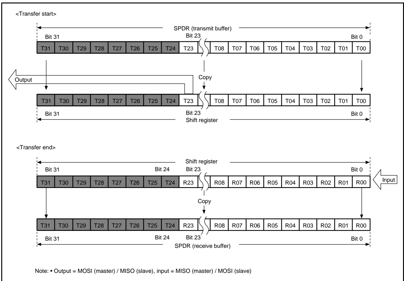
Figure 35.16 MSB-First Transfer (24-Bit Data, Parity Disabled)
