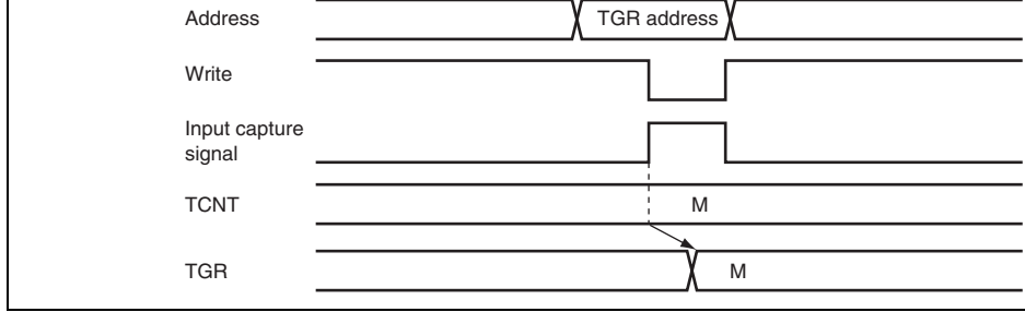
Figure 10.51 Conflict between TGR Write and Input Capture
