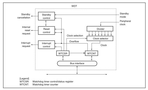
Figure 12.1 Block Diagram of WDT
