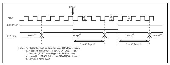
Figure 13.9 STATUS Output When Sleep Mode is Canceled by a Manual Reset
