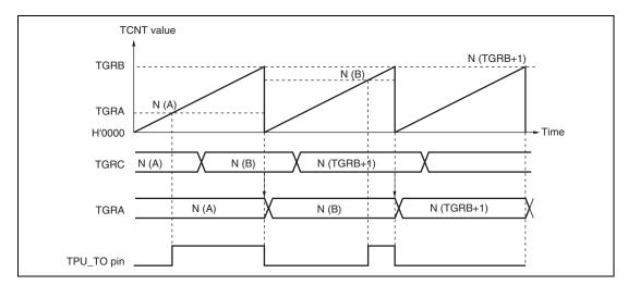
Figure 15.10 Example of Buffer Operation
