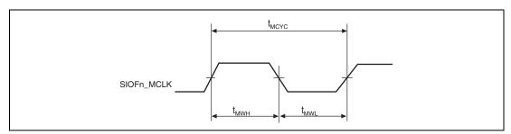
Figure 38.53 SIOF\_MCLK Input Timing
