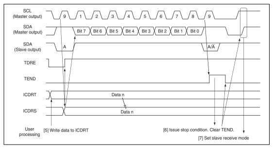
Figure 20.6 Master Transmit Mode Operation Timing (2)
