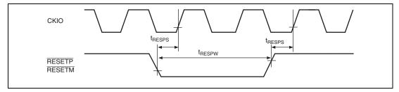
Figure 38.8 Reset Input Timing
