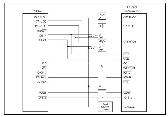
Figure 9.37 Example of PCMCIA Interface Connection
