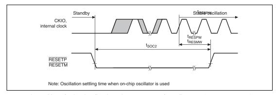
Figure 38.5 Oscillation Settling Time on Return from Standby (Return by Reset)
