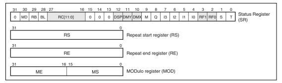
Figure 3.2 CPU Registers in DSP Mode
