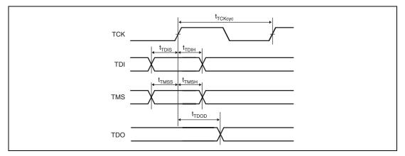
Figure 38.67 H-UDI Data Transfer Timing
