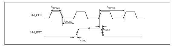
Figure 38.62 SIM Module Signal Timing
