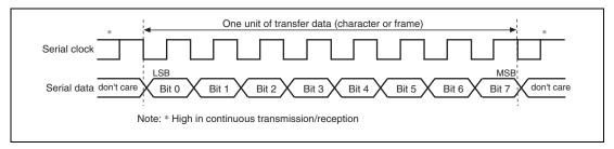
Figure 18.12 Data Format in Synchronous Communication
