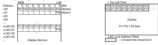
5. Packed 2bpp (Pixel Alignment in Byte is Little Endian)
