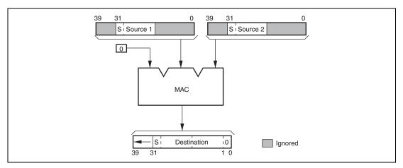
Figure 3.16 Fixed-Point Multiply Operation Flow
