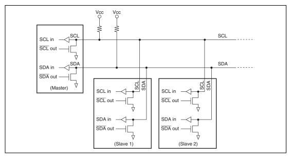
Figure 20.2 External Circuit Connections of I/O Pins
