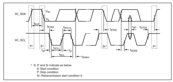
Figure 38.52 I<sup>2</sup>C Bus Interface Input/Output Timing
