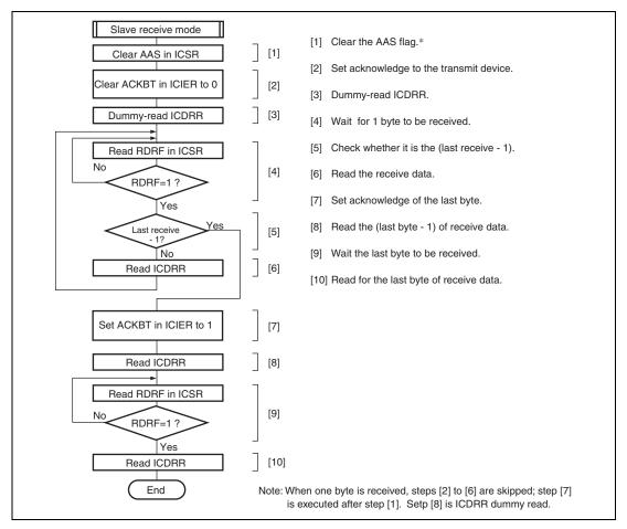
Figure 20.17 Sample Flowchart for Slave Receive Mode
