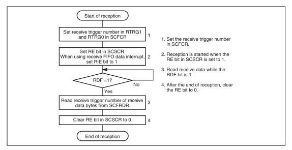
Figure 18.15 Sample Serial Reception Flowchart (1) (First Reception after Initialization)
