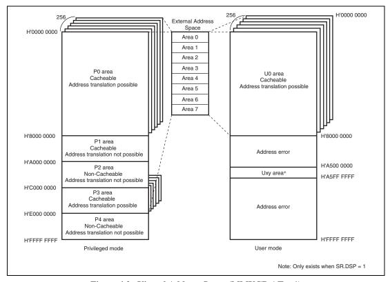
Figure 4.2 Virtual Address Space (MMUCR.AT = 1)
