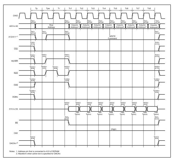
Figure 38.33 Burst Write Bus Cycle of SDRAM (Single Write  $\times$  8) (Bank Active Mode: PRE + ACTV + WRIT Command, TRCD = 1 Cycle)
