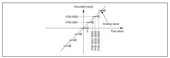
Figure 3.21 Definition of Rounding Operation
