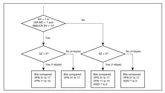
Figure 4.10 Objects of Address Comparison
