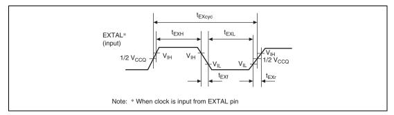
Figure 38.1 EXTAL Clock Input Timing
