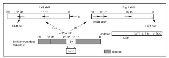
Figure 3.17 Arithmetic Shift Operation Flow
