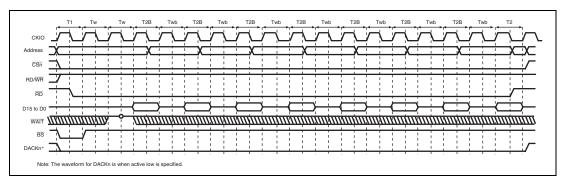
Figure 9.44 Burst ROM (Clock Synchronous) Access Timing (Burst Length = 8, Wait Cycles inserted in First Access = 2, Wait Cycles inserted in Second and Subsequent Accesses = 1)
