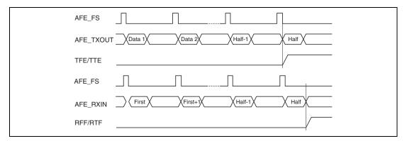
Figure 22.2 FIFO Interrupt Timing
