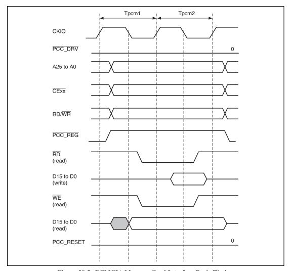
Figure 29.5 PCMCIA Memory Card Interface Basic Timing
