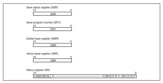
Figure 2.6 Control Register Configuration
