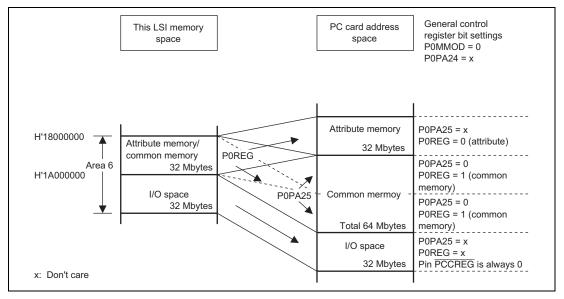
Figure 29.2 Continuous 32-Mbyte Area Mode
