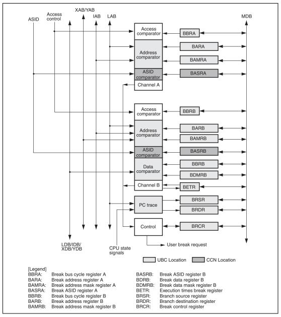
Figure 33.1 Block Diagram of UBC
