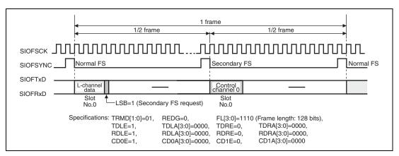
Figure 21.8 Control Data Interface (Secondary FS)
