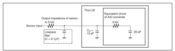
Figure 27.8 Analog Input Circuit Example
