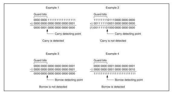
Figure 3.11 DC Bit Generation Examples in Carry or Borrow Mode
