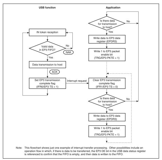
Figure 25.13 EP3 Interrupt-In Transfer Operation
