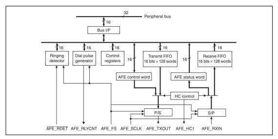
Figure 22.1 Block Diagram of AFE Interface
