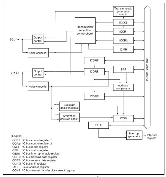
Figure 20.1 Block Diagram of I<sup>2</sup>C Bus Interface
