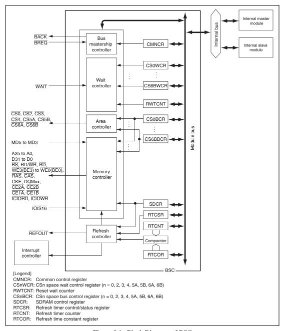
Figure 9.1 Block Diagram of BSC
