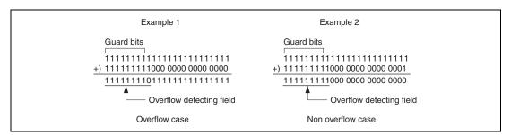
Figure 3.13 DC Bit Generation Examples in Overflow Mode
