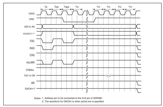
Figure 9.30 Transition Timing in Deep Power-Down Mode
