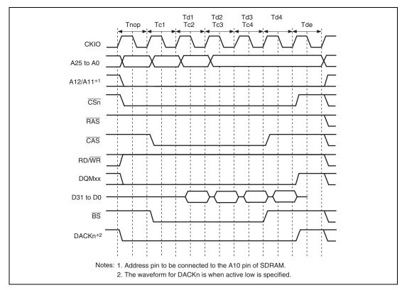
Figure 9.20 Burst Read Timing (Bank Active, Same Row Address)
