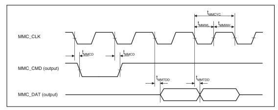
Figure 38.63 MMCIF Transmit Timing
