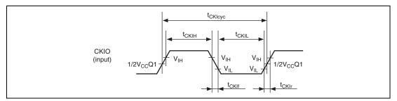
Figure 38.3 CKIO Clock Input Timing
