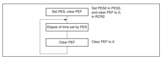
Figure 17.5 Using Periodic Interrupt Function
