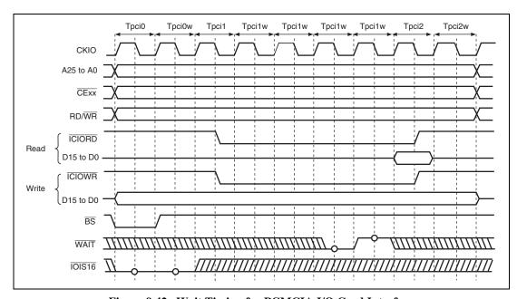
Figure 9.42 Wait Timing for PCMCIA I/O Card Interface (TED[3:0] = B'0010, TEH[3:0] = B'0001, Software Wait = 1, Hardware Wait = 1)
