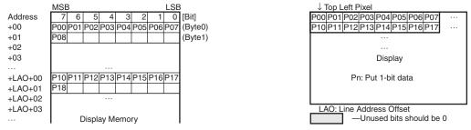
2. Packed 2bpp (Pixel Alignment in Byte is Big Endian) [Windows CE Recommended Format]
