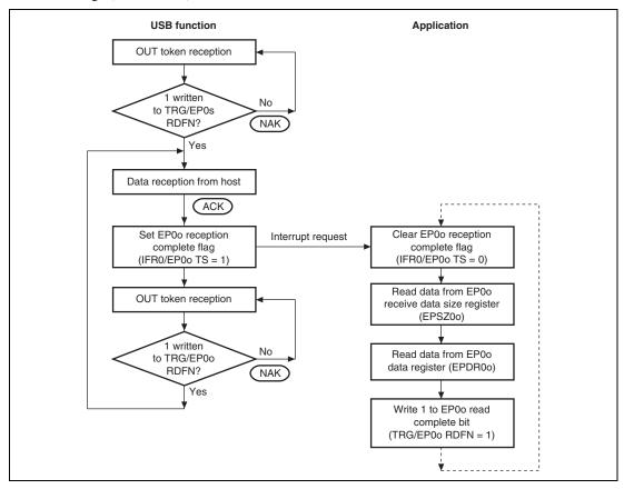
Figure 25.8 Data Stage (Control-Out) Operation
