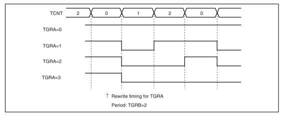
Figure 15.13 Examples of PWM Mode Operation (2)
