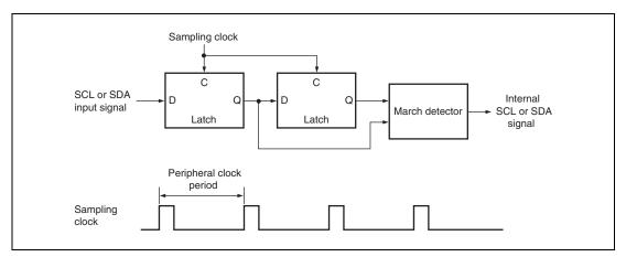
Figure 20.13 Block Diagram of Noise Conceller
