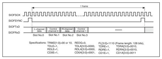
Figure 21.7 Control Data Interface (Slot Position)
