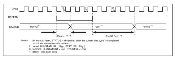
Figure 13.3 STATUS Output at Manual Reset
