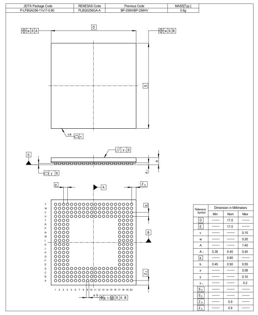
Figure C.1 Package Dimensions (PLBG0256GA-A (BP-256H/HV))
