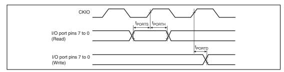
Figure 38.44 I/O Port Timing
