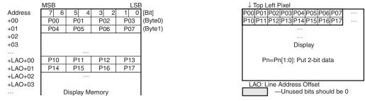
3. Packed 4bpp (Pixel Alignment in Byte is Big Endian) [Windows CE Recommended Format]
