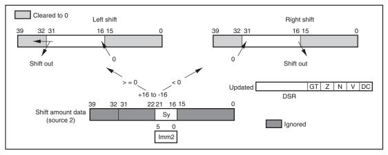
Figure 3.18 Logical Shift Operation Flow
