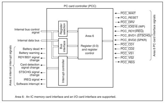
Figure 29.1 PC Card Controller Block Diagram
