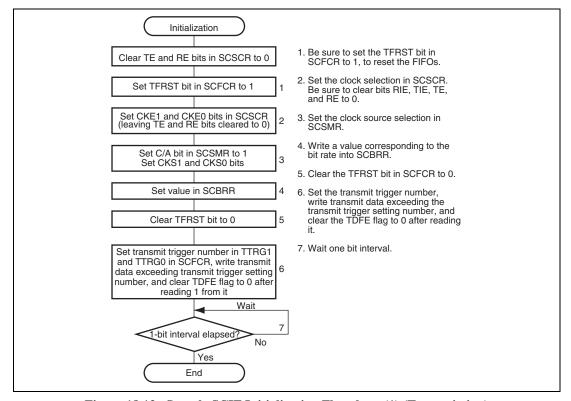
Figure 18.13 Sample SCIF Initialization Flowchart (1) (Transmission)
