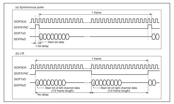
Figure 21.3 Serial Data Synchronization Timing
