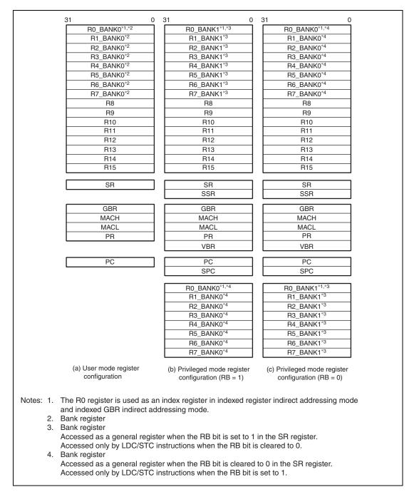
Figure 2.3 Register Configuration in Each Processing Mode
