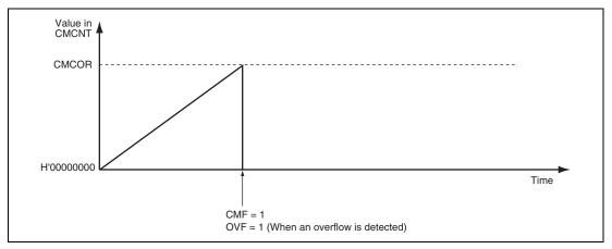
Figure 16.2 Counter Operation (One-Shot Operation)
