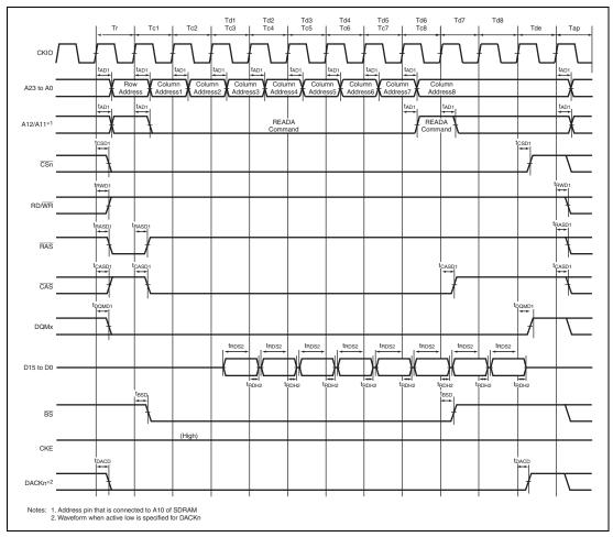
Figure 38.22 Burst Read Bus Cycle of SDRAM (Single Read  $\times$  8) (Auto Precharge Mode, CAS Latency 2, TRCD = 1 Cycle, TRP = 2 Cycles)
