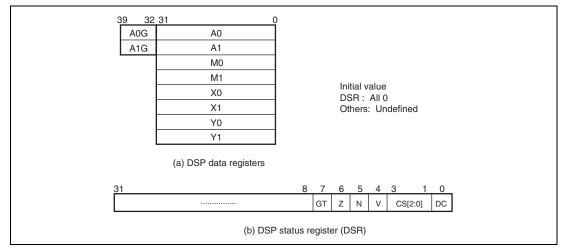
Figure 3.3 DSP Register Configuration
