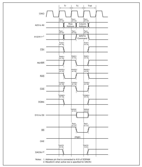
Figure 38.24 Single Write Bus Cycle of SDRAM (Auto Precharge Mode, TRWL = 1 Cycle)
