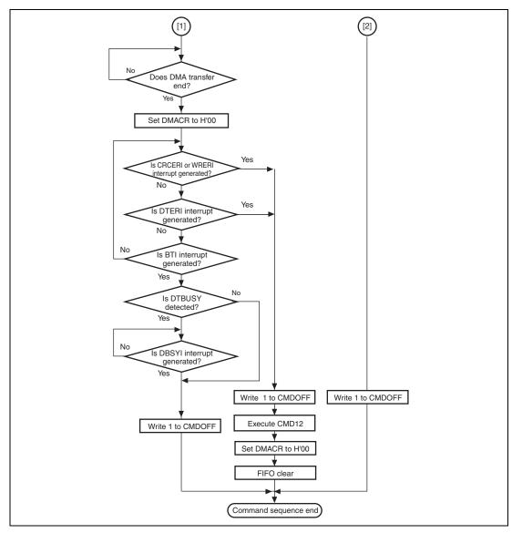
Figure 31.32 Operational Flowchart for Pre-defied Multiblock Write Transfer in Auto Mode (2)
