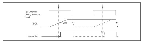
Figure 20.18 The Timing of the Bit Synchronous Circuit
