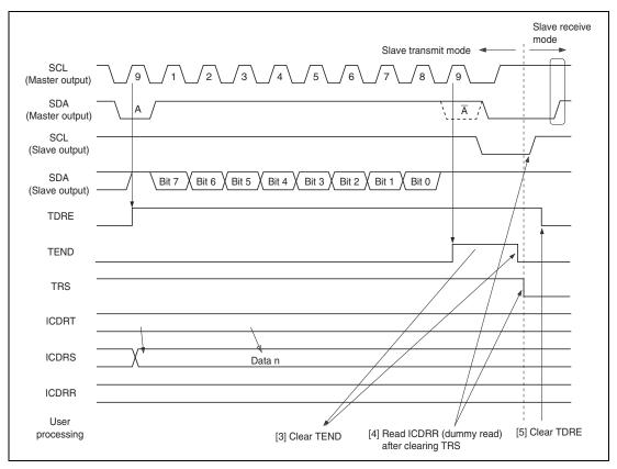
Figure 20.10 Slave Transmit Mode Operation Timing (2)
