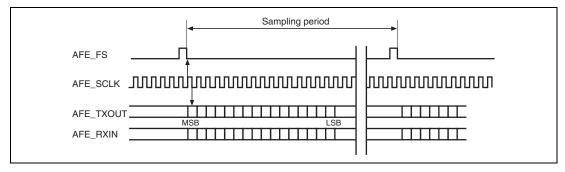
Figure 22.5 AFE Serial Interface
