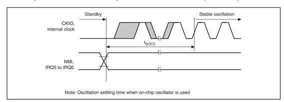
Figure 38.6 Oscillation Settling Time on Return from Standby (Return by NMI or IRQ)
