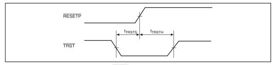
Figure 38.66 TRST Input Timing (Reset Hold)
