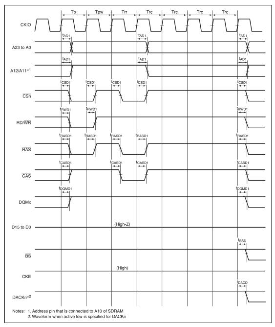
Figure 38.34 Auto Refresh Timing of SDRAM (TRP = 2 Cycles)
