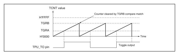
Figure 15.7 Example of Toggle Output Operation
