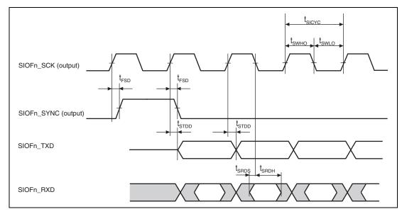
Figure 38.54 SIOF Transmission/Reception Timing (Master Mode 1, Fall Sampling)
