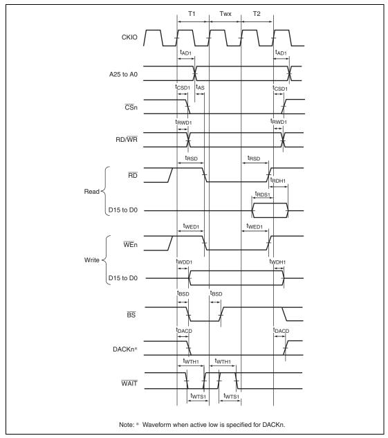
Figure 38.14 Basic Bus Cycle in Normal Space (External Wait 1 Input)
