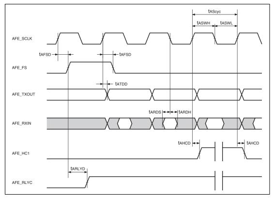
Figure 38.59 AFEIF Module AC Timing
