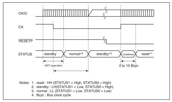
Figure 13.11 Hardware Standby Mode Timing (CA is pulled low while WDT operates after the standby mode is canceled)
