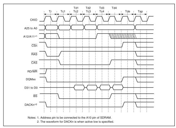
Figure 9.14 Burst Read Basic Timing (Auto-Precharge)
