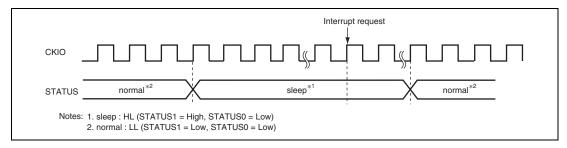
Figure 13.7 STATUS Output when Sleep Mode is Canceled by an Interrupt
