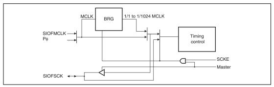
Figure 21.2 Serial Clock Supply
