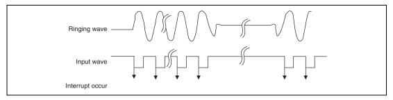
Figure 22.3 Ringing Interrupt Occurrence Timing
