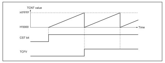
Figure 15.3 Free-Running Counter Operation
