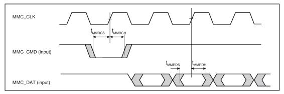
Figure 38.64 MMCIF Receive Timing (Rise Sampling)
