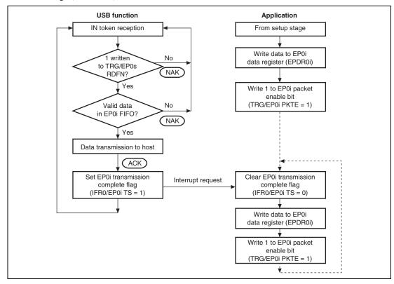
Figure 25.7 Data Stage (Control-In) Operation
