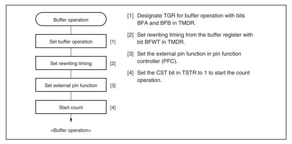
Figure 15.9 Example of Buffer Operation Setting Procedure
