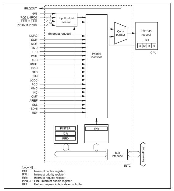
Figure 8.1 Block Diagram of INTC
