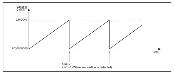
**Figure 16.3 Counter Operation (Free-Running Operation)**
