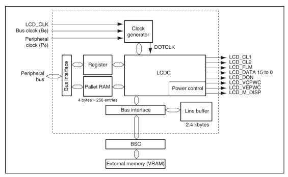
Figure 26.1 LCDC Block Diagram
