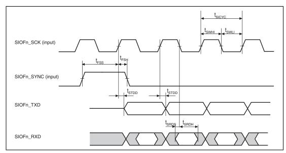
Figure 38.58 SIOF Transmission/Reception Timing (Slave Mode 1, Slave Mode 2)
