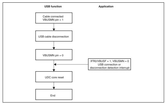
Figure 25.4 Cable Disconnection Operation
