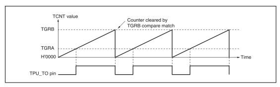
Figure 15.12 Example of PWM Mode Operation (1)
