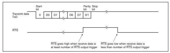
Figure 18.11 Example of RTS Control Operation
