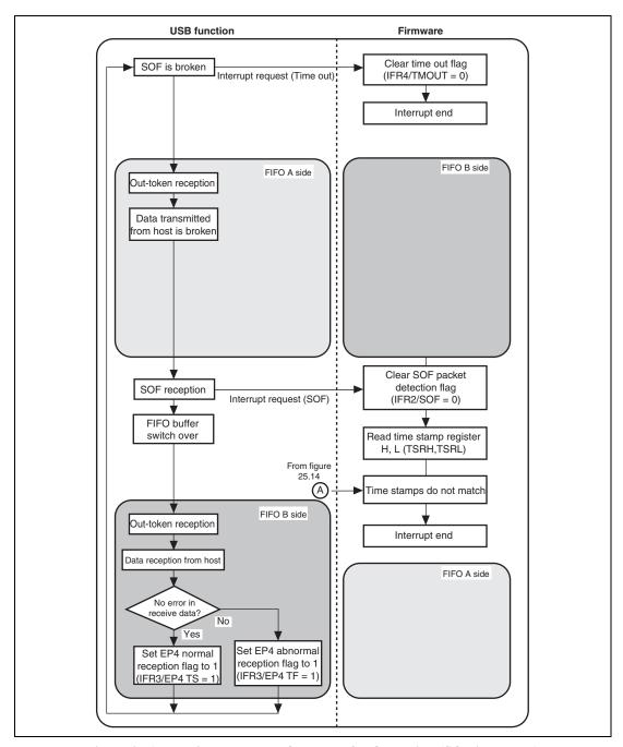
Figure 25.15 EP4 Isochronous-Out Transfer Operation (SOF is Broken)
