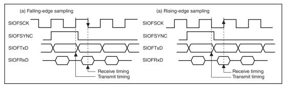
Figure 21.4 SIOF Transmit/Receive Timing
