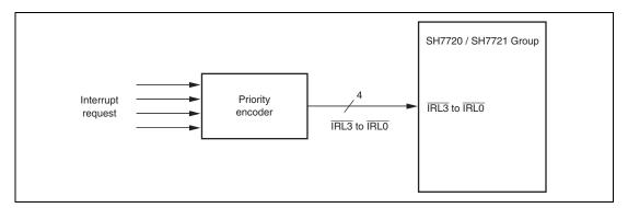
Figure 8.2 Example of IRL Interrupt Connection
