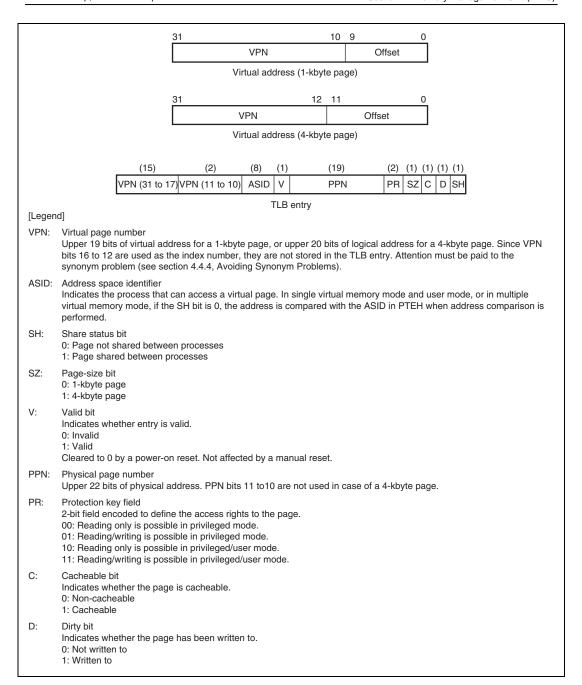
Figure 4.7 Virtual address and TLB Structure
