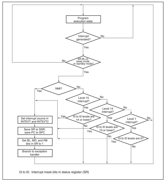
Figure 8.3 Interrupt Operation Flowchart
