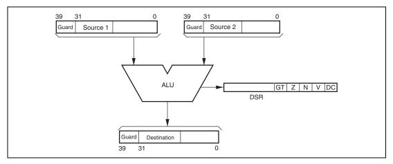
Figure 3.9 ALU Fixed-Point Arithmetic Operation Flow
