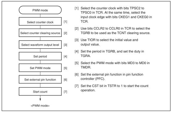
Figure 15.11 Example of PWM Mode Setting Procedure
