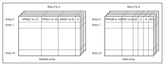
Figure 4.6 Overall Configuration of the TLB
