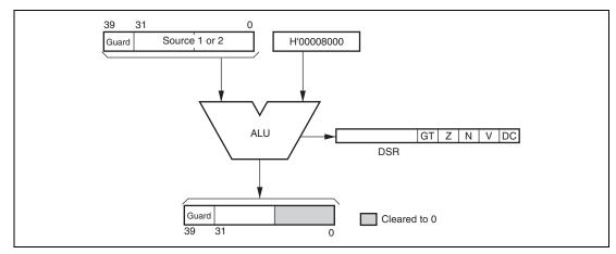
Figure 3.20 Rounding Operation Flow
