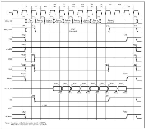
Figure 38.28 Burst Read Bus Cycle of SDRAM (Single Read  $\times$  8) (Bank Active Mode: ACTV + READ Command, CAS Latency 2, TRCD = 1 Cycle)
