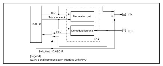
Figure 19.1 Block Diagram of IrDA
