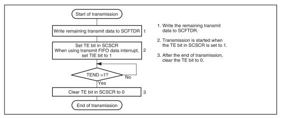
Figure 18.14 Sample Serial Transmission Flowchart (1) (First Transmission after Initialization)
