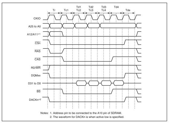
Figure 9.19 Burst Read Timing (No Auto-Precharge)
