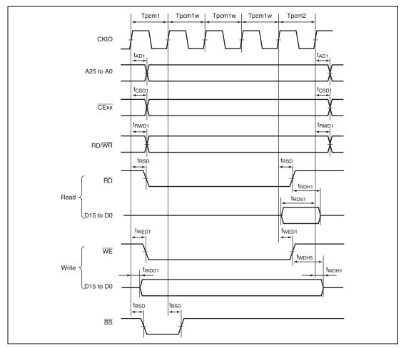
Figure 38.39 PCMCIA Memory Card Interface Bus Timing
