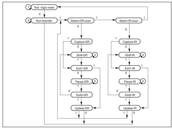
Figure 36.2 TAP Controller State Transitions
