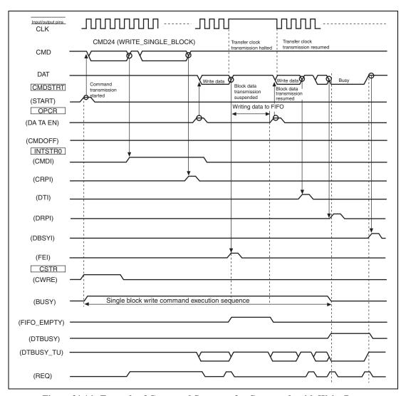
Figure 31.16 Example of Command Sequence for Commands with Write Data (Block Size > FIFO Size)
