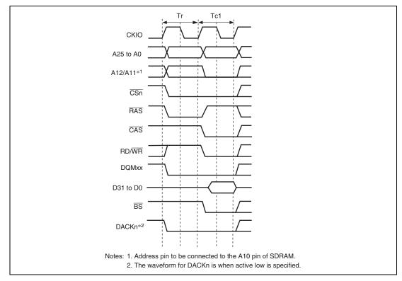
Figure 9.22 Single Write Timing (No Auto-Precharge)
