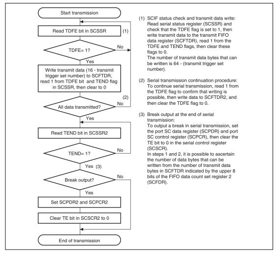
Figure 18.3 Sample Serial Transmission Flowchart
