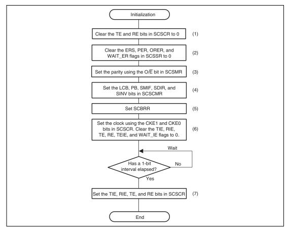
Figure 30.4 Example of Initialization Flow
