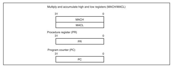
Figure 2.5 System Registers and Program Counter
