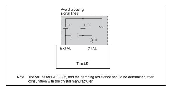
Figure 11.2 Points for Attention when Using Crystal Resonator
