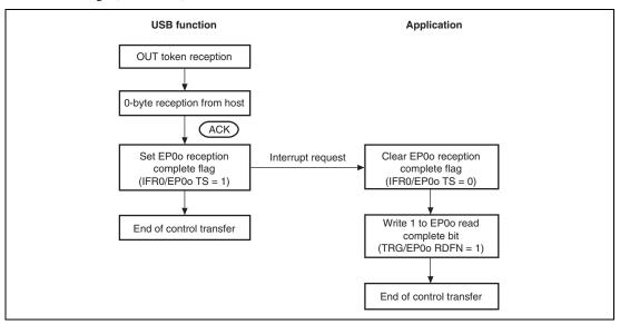
Figure 25.9 Status Stage (Control-In) Operation
