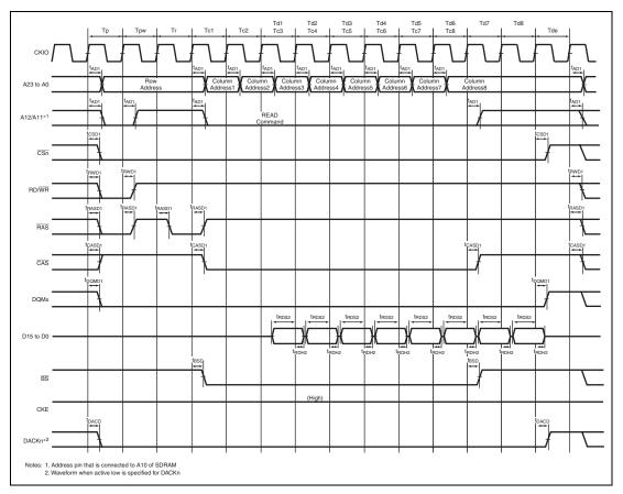
Figure 38.30 Burst Read Bus Cycle of SDRAM (Single Read × 8)
