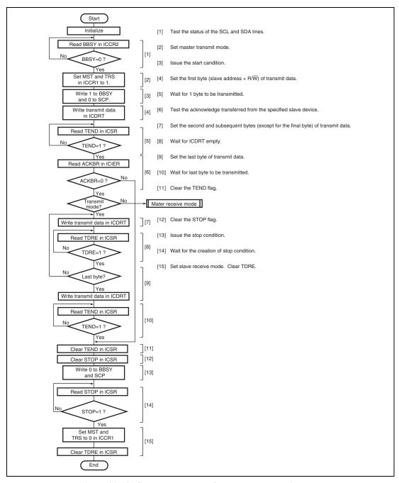
Figure 20.14 Sample Flowchart for Master Transmit Mode
