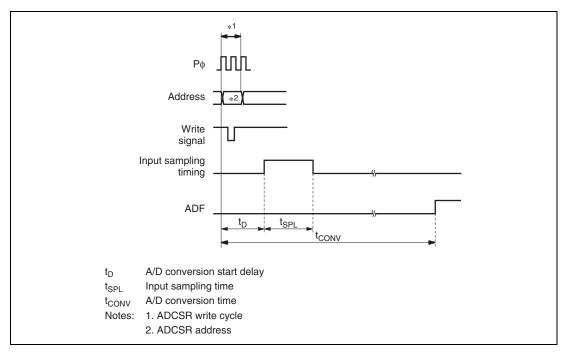
Figure 27.5 A/D Conversion Timing
