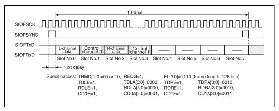
Figure 21.19 Transmit and Receive Timing (16-Bit Stereo Data (4))
