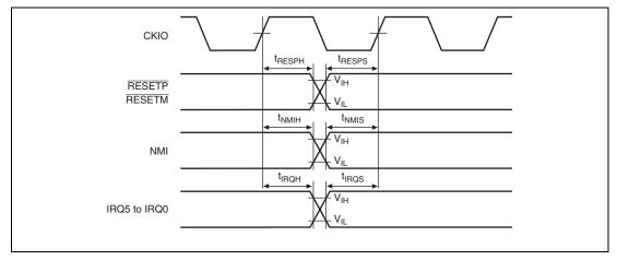
Figure 38.9 Interrupt Signal Input Timing
