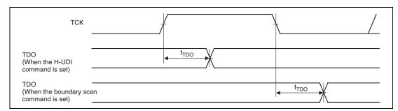
Figure 36.3 H-UDI Data Transfer Timing
