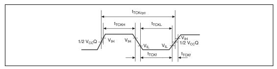
Figure 38.65 TCK Input Timing
