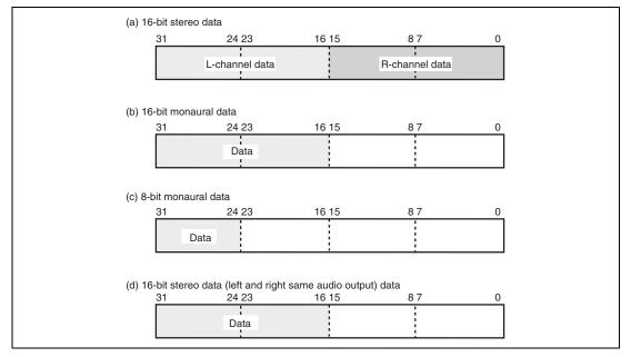
Figure 21.5 Transmit/Receive Data Bit Alignment
