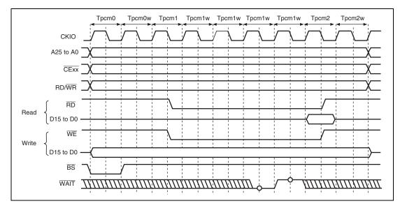
Figure 9.39 Wait Timing for PCMCIA Memory Card Interface (TED[3:0] = B'0010, TEH[3:0] = B'0001, Software Wait = 1, Hardware Wait = 1)
