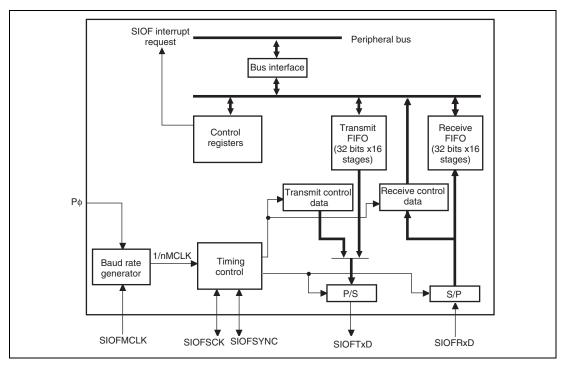
Figure 21.1 Block Diagram of SIOF
