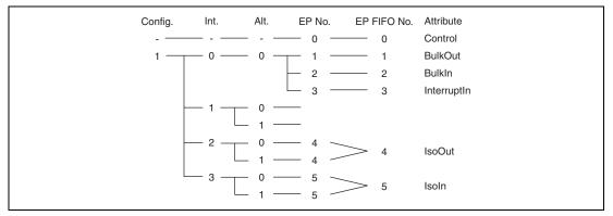
Figure 25.2 Example of Endpoint Configuration
