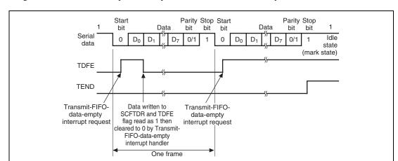
Figure 18.4 shows an example of the operation for transmission in asynchronous mode.
