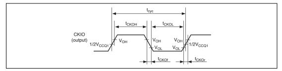
Figure 38.2 CKIO Clock Output Timing
