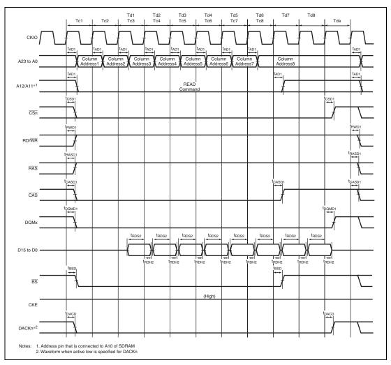
Figure 38.29 Burst Read Bus Cycle of SDRAM (Single Read × 8)
