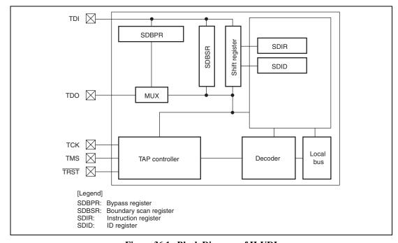
Figure 36.1 Block Diagram of H-UDI
