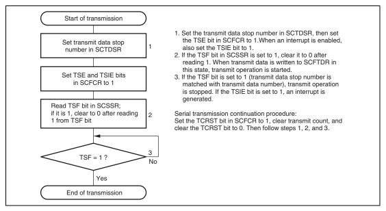
Figure 18.6 Transmit Data Stop Function Flowchart
