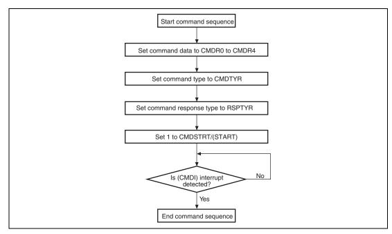
Figure 31.3 Operational Flow for Commands that do not Require Command Response
