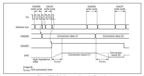
Figure 28.2 D/A Converter Operation Example
