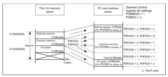
Figure 29.3 Continuous 16-Mbyte Area Mode (Area 6)
