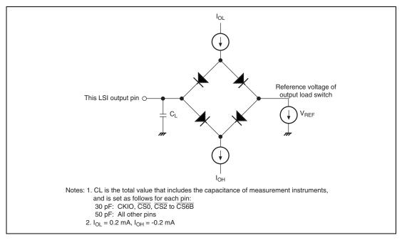
Figure 38.69 Output Load Circuit
