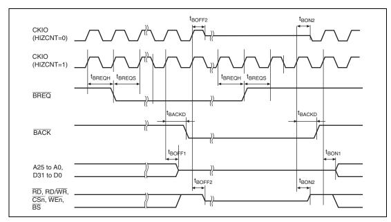
Figure 38.10 Bus Release Timing
