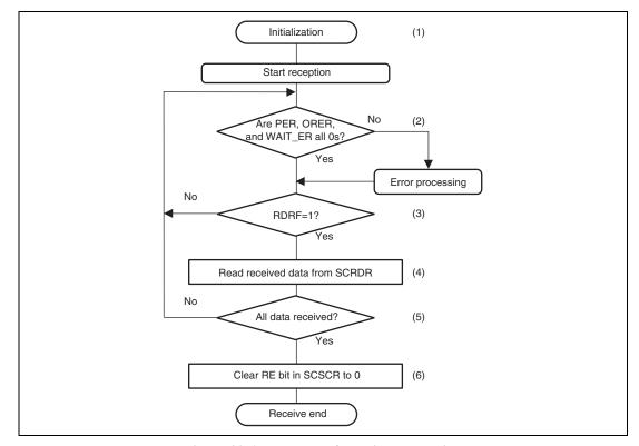
Figure 30.6 Example of Receive Processing
