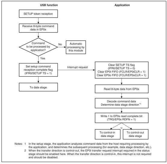
Figure 25.6 Setup Stage Operation
