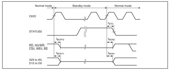
Figure 38.11 Pin Drive Timing at Standby
