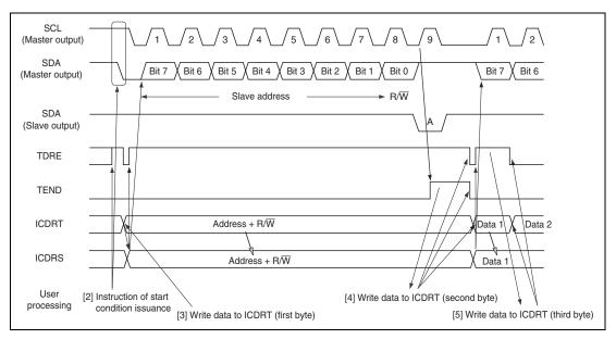
Figure 20.5 Master Transmit Mode Operation Timing (1)
