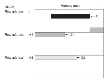
In above figure, transfer data 1 and 3 are able to be read or written by USB Host Controller. But transfer data 2 are possibly unable to be read or written by USB Host controller. Any data, which have possibility to be accessed by USB Host Controller, must be aligned in SDRAM not to cross row address alignment.
