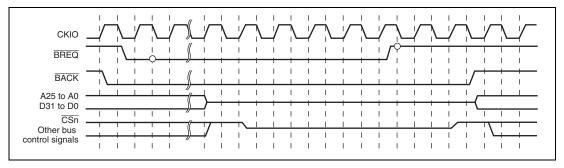
Figure 9.45 Bus Arbitration Timing
