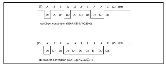
Figure 30.3 Examples of Start Character Waveforms
