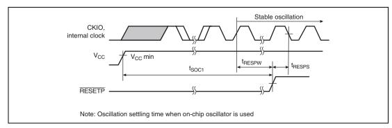
Figure 38.4 Power-On Oscillation Settling Time
