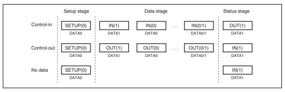
Figure 25.5 Transfer Stages in Control Transfer
