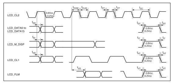
Figure 38.61 LCDC Module Signal Timing
