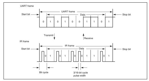
Figure 19.2 Transmit/Receive Operation
