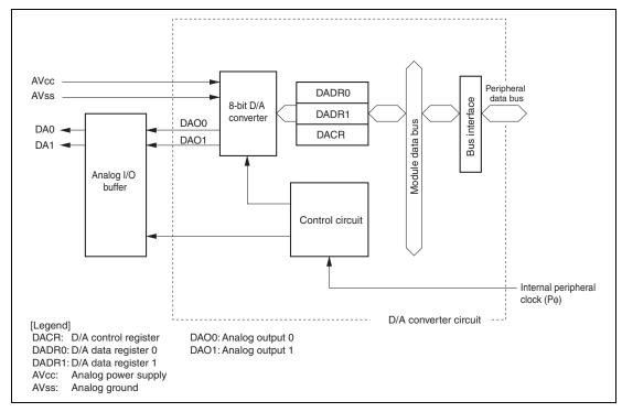
Figure 28.1 Block Diagram of D/A Converter
