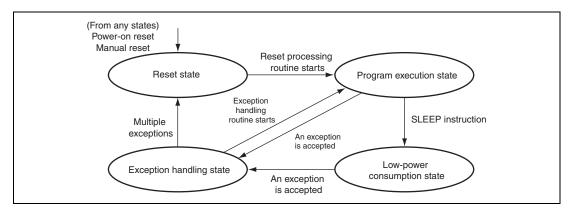
Figure 2.1 Processing State Transitions
