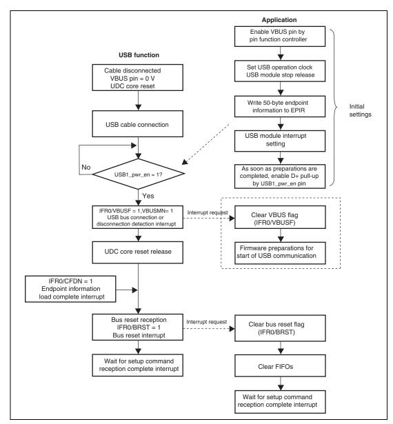
Figure 25.3 Cable Connection Operation
