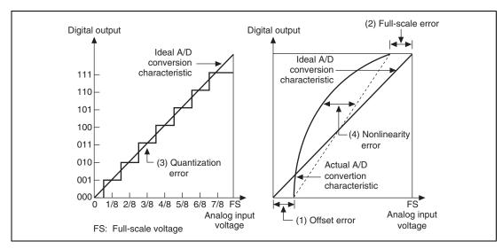
Figure 27.7 Definitions of A/D Conversion Accuracy
