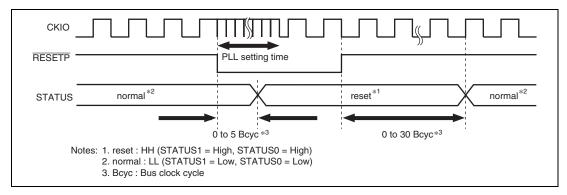
Figure 13.2 STATUS Output at Power-on Reset
