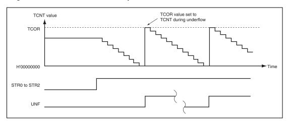
Figure 14.3 Auto-Reload Count Operation
