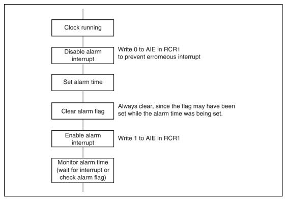
Figure 17.4 Using Alarm Function
