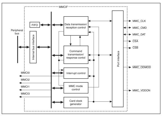
Figure 31.1 Block Diagram of MMCIF
