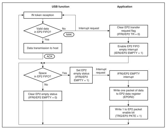
Figure 25.12 EP2 Bulk-In Transfer Operation
