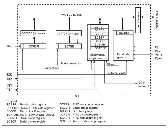
Figure 18.1 Block Diagram of SCIF
