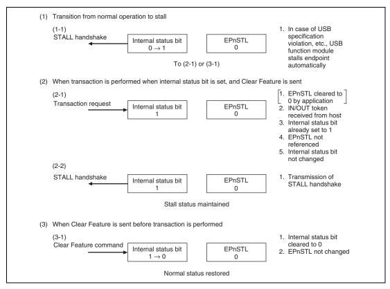
Figure 25.19 Automatic Stall by USB Function Controller
