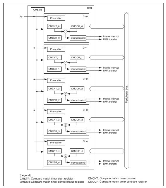
Figure 16.1 Block Diagram of CMT
