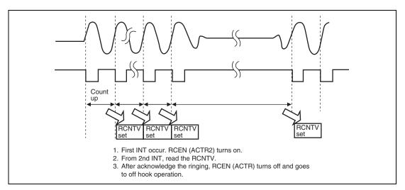
Figure 22.8 Ringing Detect Sequence
