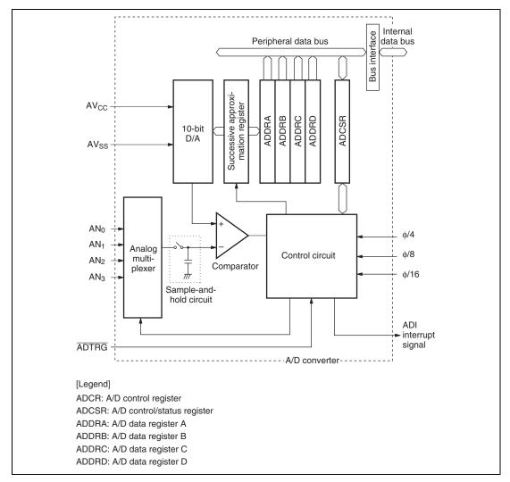
Figure 27.1 Block Diagram of A/D Converter
