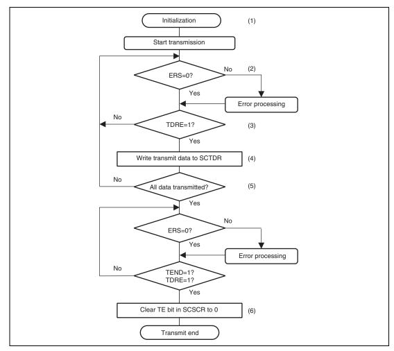
Figure 30.5 Example of Transmit Processing
