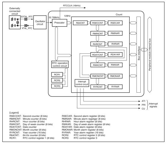
Figure 17.1 RTC Block Diagram
