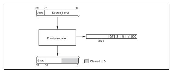
Figure 3.19 PDMSB Operation Flow
