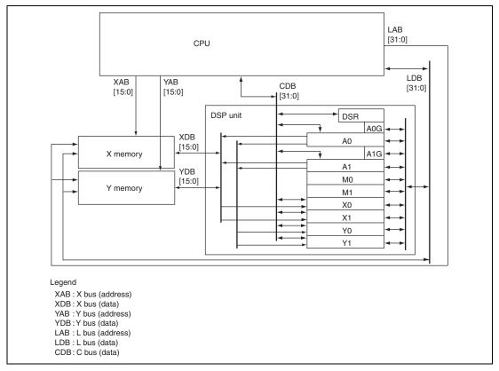
Figure 3.4 DSP Registers and Bus Connections
