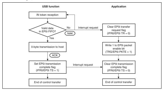
Figure 25.10 Status Stage (Control-Out) Operation
