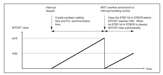
Figure 13.1 Canceling Standby Mode with STBY Bit in STBCR
