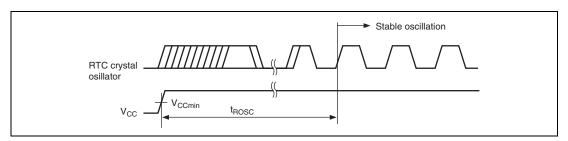
Figure 38.49 Oscillation Settling Time when RTC Crystal Oscillator is Turned On
