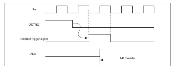
Figure 27.6 External Trigger Input Timing
