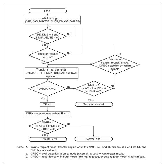
Figure 10.2 DMA Transfer Flowchart
