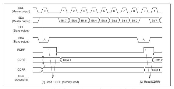
Figure 20.11 Slave Receive Mode Operation Timing (1)
