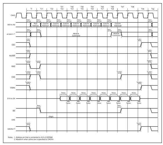
Figure 38.23 Burst Read Bus Cycle of SDRAM (Single Read  $\times$  8) (Auto Precharge Mode, CAS Latency 2, TRCD = 2 Cycles, TRP = 1 Cycle)
