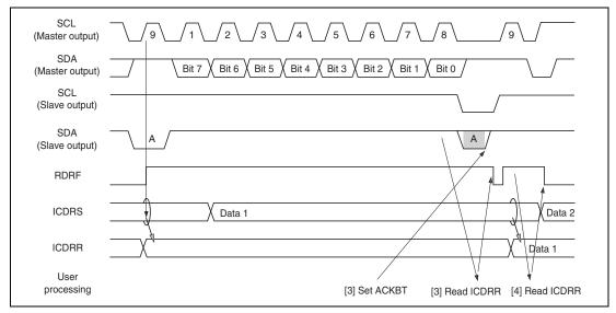
Figure 20.12 Slave Receive Mode Operation Timing (2)
