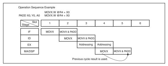
Figure 3.10 Operation Sequence Example
