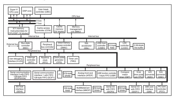
Figure 1.1 Block Diagram
