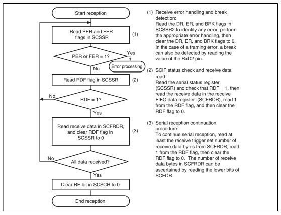
Figure 18.7 Sample Serial Reception Flowchart (1)
