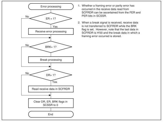
Figure 18.8 Sample Serial Reception Flowchart (2)
