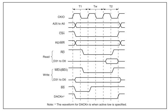
Figure 9.9 Wait Timing for Normal Space Access (Software Wait Only)
