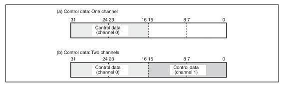
Figure 21.6 Control Data Bit Alignment
