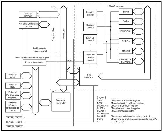
Figure 10.1 Block Diagram of DMAC
