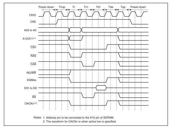
Figure 9.27 Access Timing in Power-Down Mode
