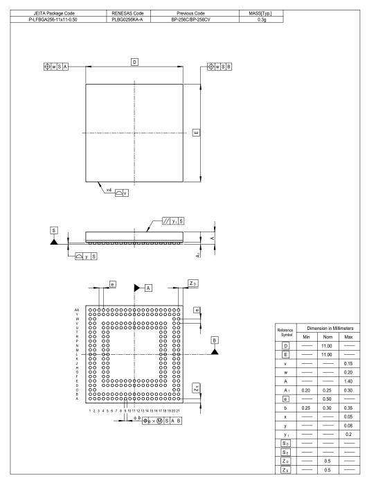
Figure C.2 Package Dimensions (PLBG0256KA-A (BP-256C/CV))
