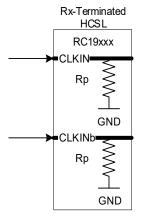
Figure 17. Receiver Termination
