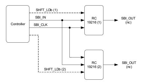
Figure 28. Side-Band Interface Star Topology
