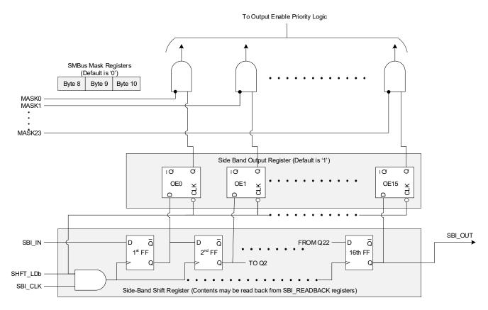
Figure 24. Side-band Interface High-Level Functional Diagram (RC192xx shown)
