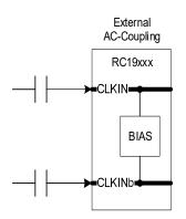
Figure 16. External AC-Coupling
