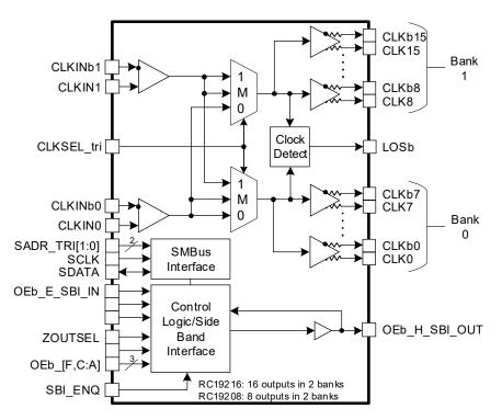
Figure 2. RC19216/RC19208 Block Diagram
