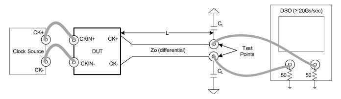
Figure 12. AC/DC Test Load for Differential Outputs (Double-Terminated)
