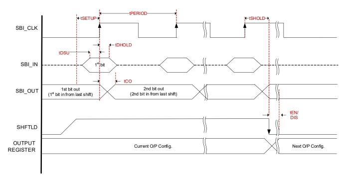
Figure 10. Side-Band Interface Timing
