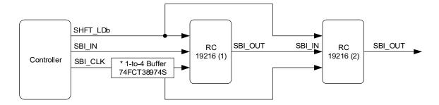
Figure 29. Side-Band Interface Daisy-Chain Topology
