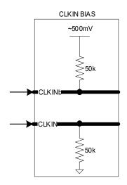
Figure 8. Clock Input Bias Network
