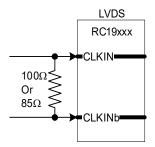
Figure 15. LVDS Input Levels
