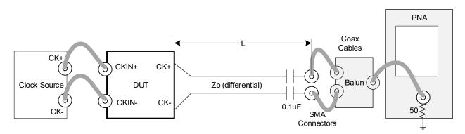
Figure 13. Test Load for PCle Phase Jitter Measurements
