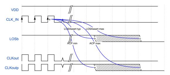
Figure 23. LOSb Assert Timing
