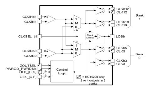
Figure 5. RC19204/RC19202 Block Diagram
