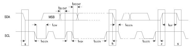
Figure 9. SMBus Slave Timing Diagram
