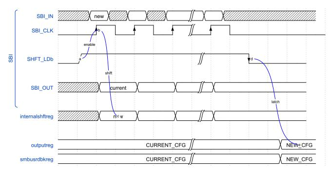
Figure 27. Side-Band Interface Functional Timing
