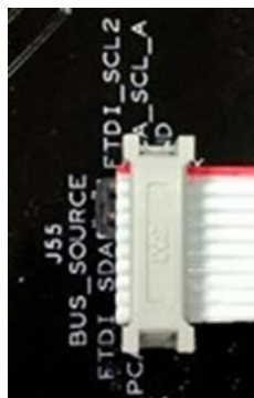
Figure 9. Aardvark Adapter Connection to J55
