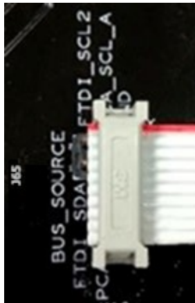
Figure 7. Aardvark Adapter Connection to J65
