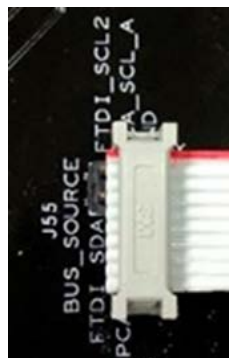
Figure 9. Aardvark Adapter Connection to J55
