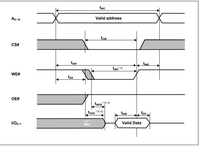
Note 14. t<sub>WP</sub> is the interval between write start and write end. A write starts when both of CS# and WE# become active. A write is performed during the overlap of a low CS# and a low WE#. A write ends when any of CS# or WE# becomes inactive.
