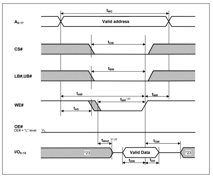
Note 20.  $t_{WP}$  is the interval between write start and write end.
