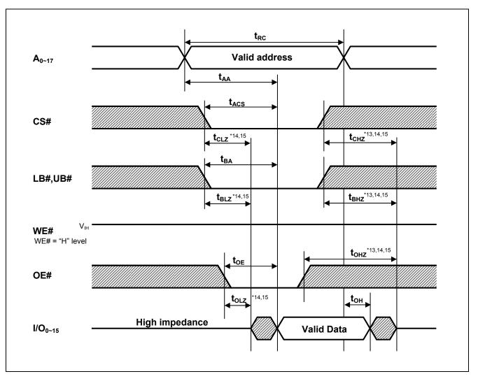
Note 13.  $t_{CHZ}$ ,  $t_{BHZ}$  and  $t_{OHZ}$  are defined as the time when the I/O pins enter a high-impedance state and are not referred to the I/O levels.
