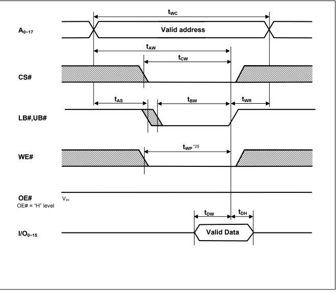
Note 25.  $t_{WP}$  is the interval between write start and write end.
