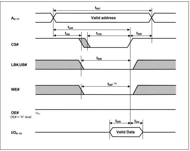
Note 24.  $t_{WP}$  is the interval between write start and write end.
