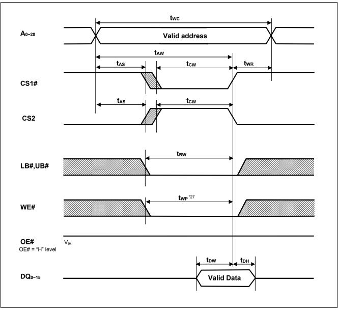
Note 27. twp is the interval between write start and write end.
