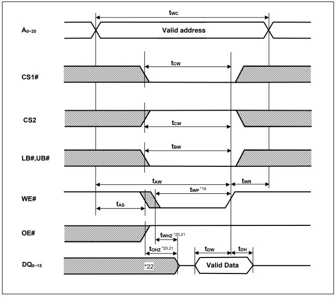
Note 19. twp is the interval between write start and write end.
