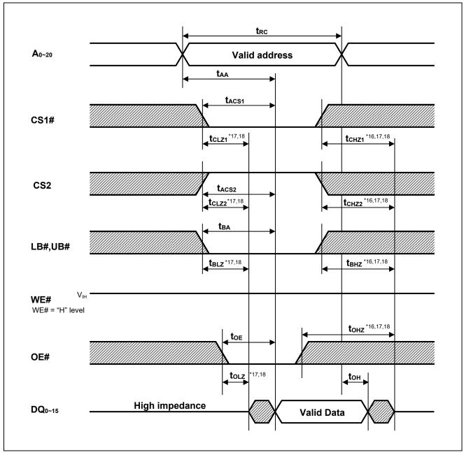
Note 16. t<sub>CHZ1</sub>, t<sub>CHZ2</sub>, t<sub>BHZ</sub> and t<sub>OHZ</sub> are defined as the time when the DQ pins enter a high-impedance state and are not referred to the DQ levels.
