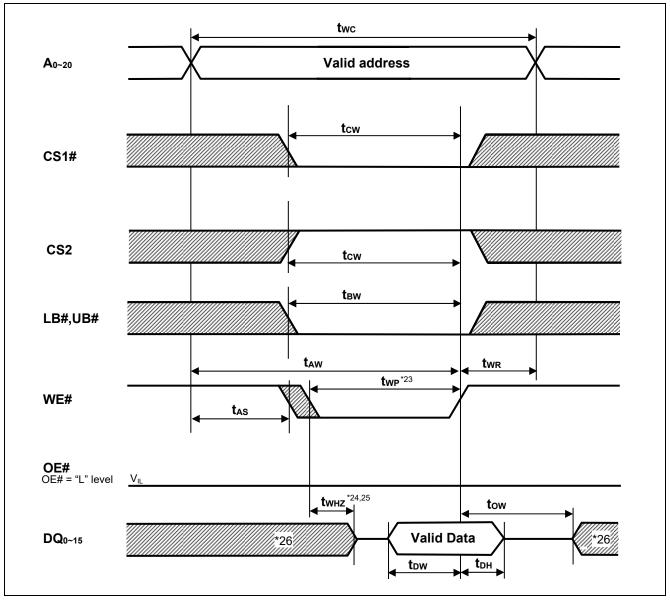
Note 23. twp is the interval between write start and write end.
