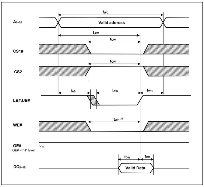
Note 28. twp is the interval between write start and write end.
