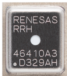
Figure 1. RRH46410 Gas Sensor
