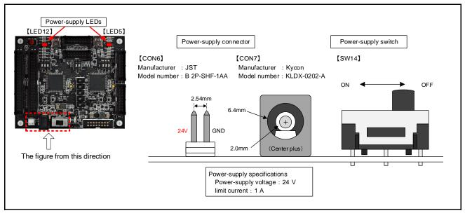
Figure 1.2.1 Power-supply Connectors and Switch
