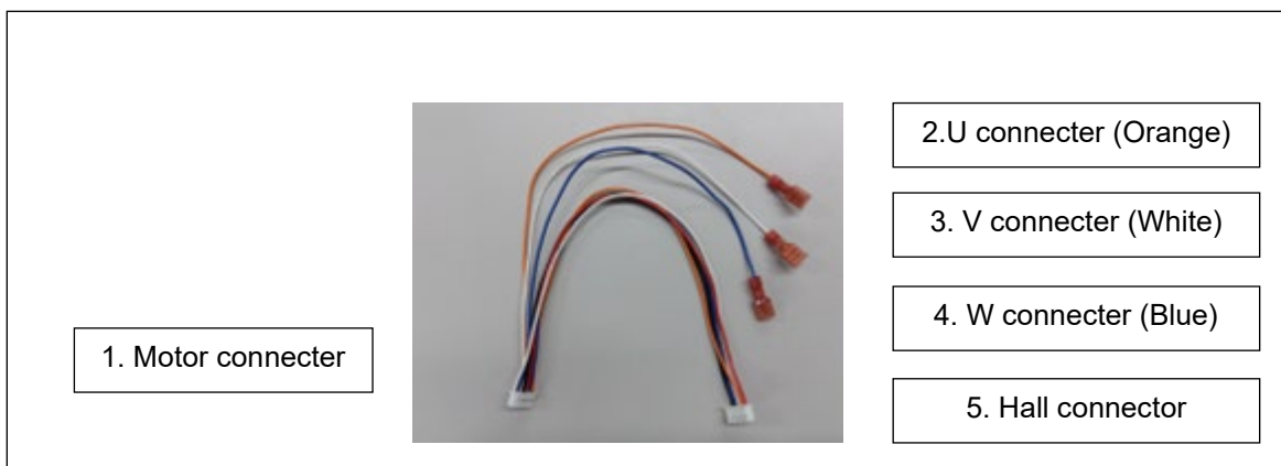
Figure 2-5 Motor Cable Connection
