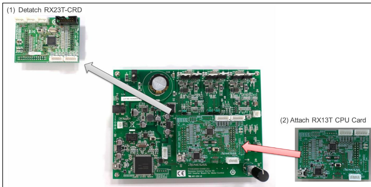
Figure 4-1 CPU card replacement
