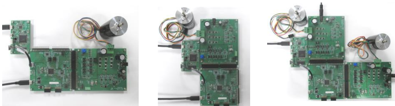
(1)CPU board + INV board (connected with CN1,CN2)
