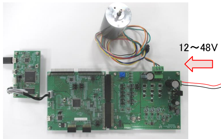
Figure 4-11 Power supply from terminal block
