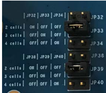
Figure 3-1 JP32/JP33/JP34/JP38/JP39/JP40 jumpers on RTK-251-1PowerBank3.
