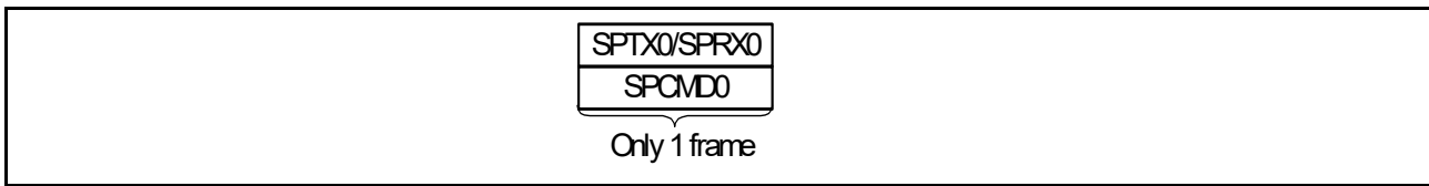
Figure 32.41 Relationship between the SPI Command Register and the transmit and receive buffers in sequence operations (SPI1)
