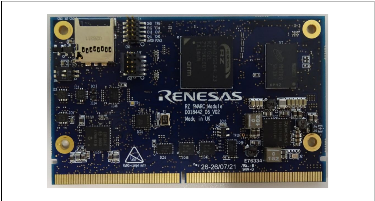
Figure 4.1 Top View of the SMARC Module Board
