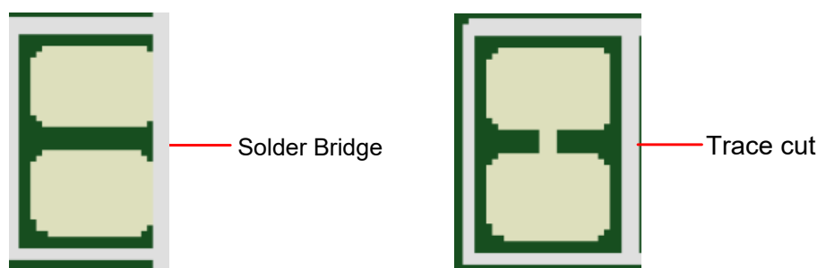
Figure 6-1 Solder Bridge and Trace Cut
