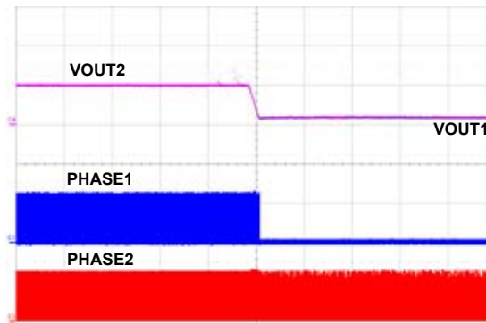
Figure 6. VOUT2 Tracking VOUT1 when Channel 1 is Disabled
