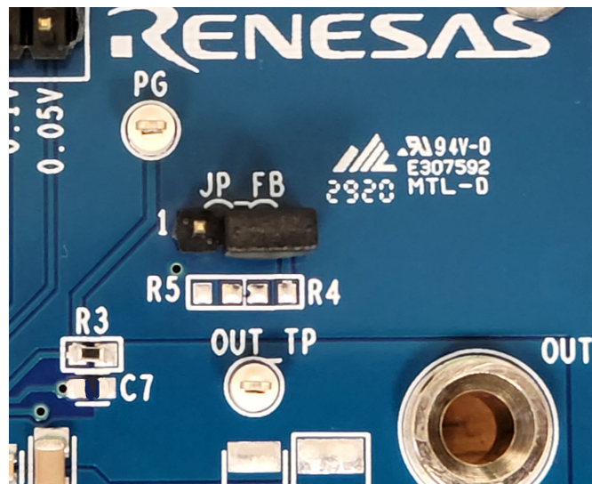
Figure 4. RTKA214023DE0000BU JP_FB Jumper for External Feedback Configuration
