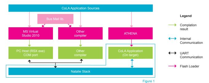
Application development can be done both on the target via an Athena environment and on the host processor as shown in figure 1.
