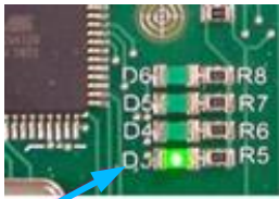
Figure 5. D3 Status LED for MCB Microcontroller
