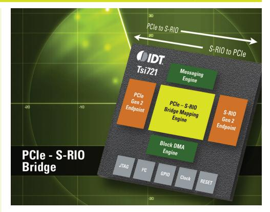
IDT is the industry's leading supplier of RapidIO® and PCI Express® Interconnect solutions, providing a broad portfolio of switches, bridges, IP and development platforms for defense, aerospace, video, imaging and wireless markets. The Tsi721 is IDT's solution for hardware based PCIe Gen 2 to RapidIO Gen 2 protocol conversion in a bridging device
